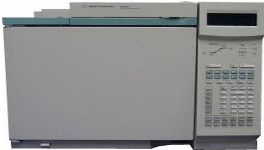
Figura 8.6 Gazkromatografi HP 6890 Series II ku u realizuan analizat e SOH me GC/ECD.
